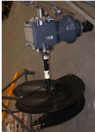
Figure 1. Auger fabrication as of Oct. 30, 2009. Shown is the auger, gear box and hydraulic drive. Not shown is the rotating steam union and 3-pt. connection.
