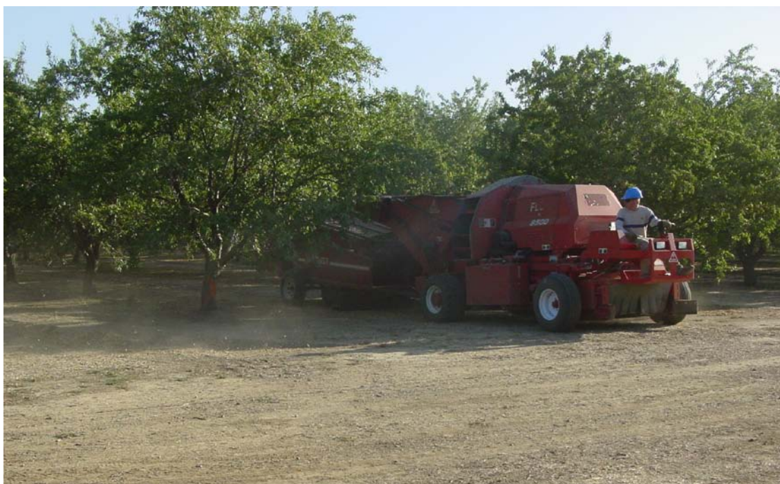
Figure 2. The conditioner unit used to test the effect of various fan suction speed on PM emissions.
