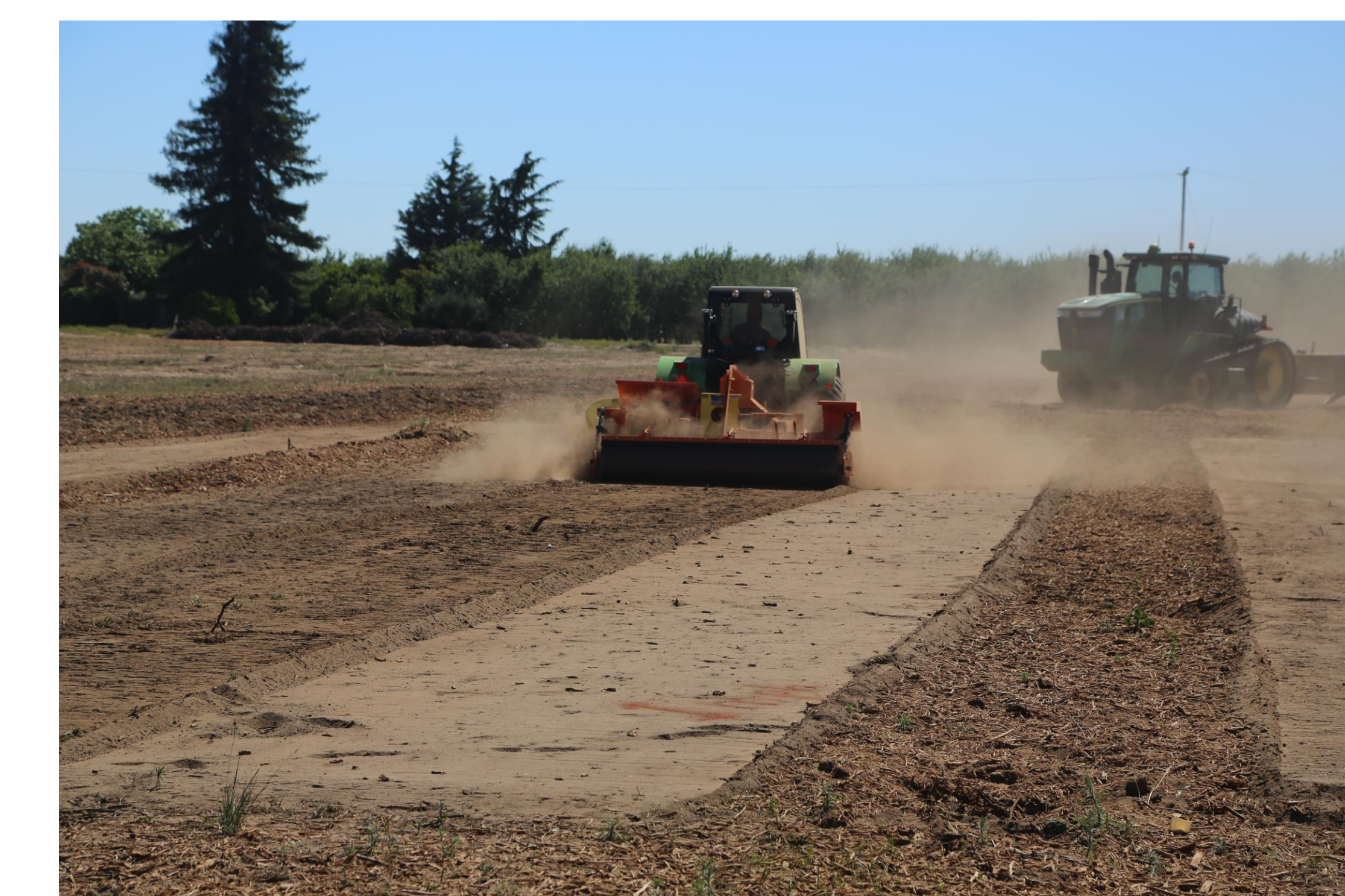
Figure 7. Northwest Tiller incorporating wood chips after they were spread on the orchard floor.
