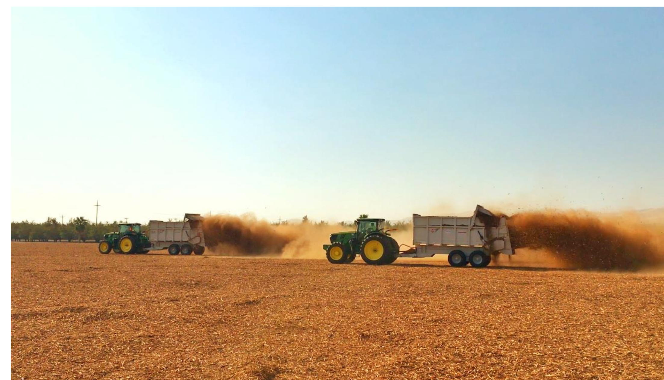
Figure 4. Kuhn & Knight Spreaders modified for spreading wood chips by G & F Ag Services in Ripon, CA.
