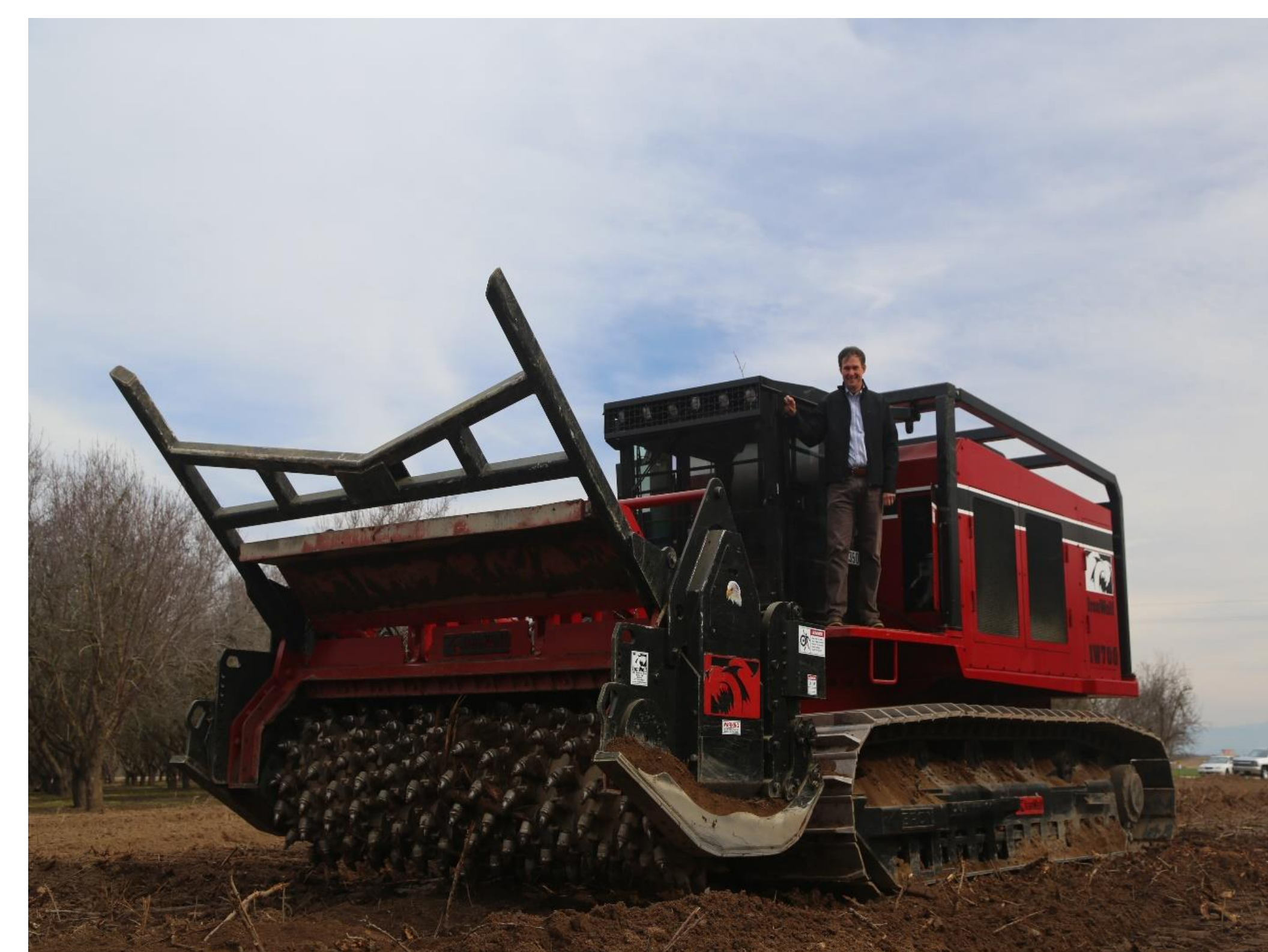
Fig. 2. The 'Iron Wolf' 700 B, a 50-ton rock crusher.
