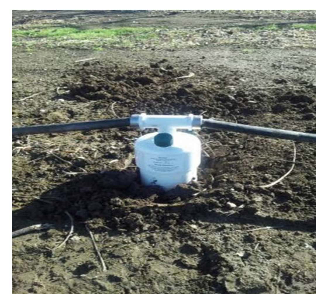
Figure 2. Microfertigation apparatus used in the HFLC subplots.
