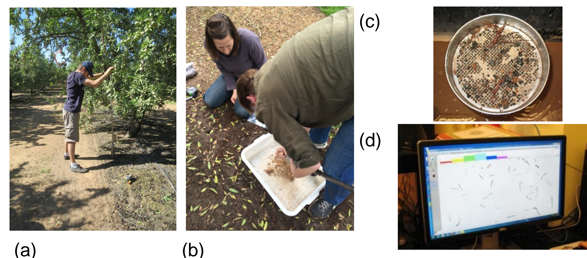
Figure 2. (a,b) Collecting soil cores at 5 consecutive soil depths (10 cm increments), (c) washing roots out of soil cores down to a sieve size of 250 \mu\text{m} , (d) scanning root length in ten 0.1 mm increment diameter size classes using WinRhizo Pro. Dry mass was measured for all samples to allow calculation of both root mass density and root length density per volume soil.
