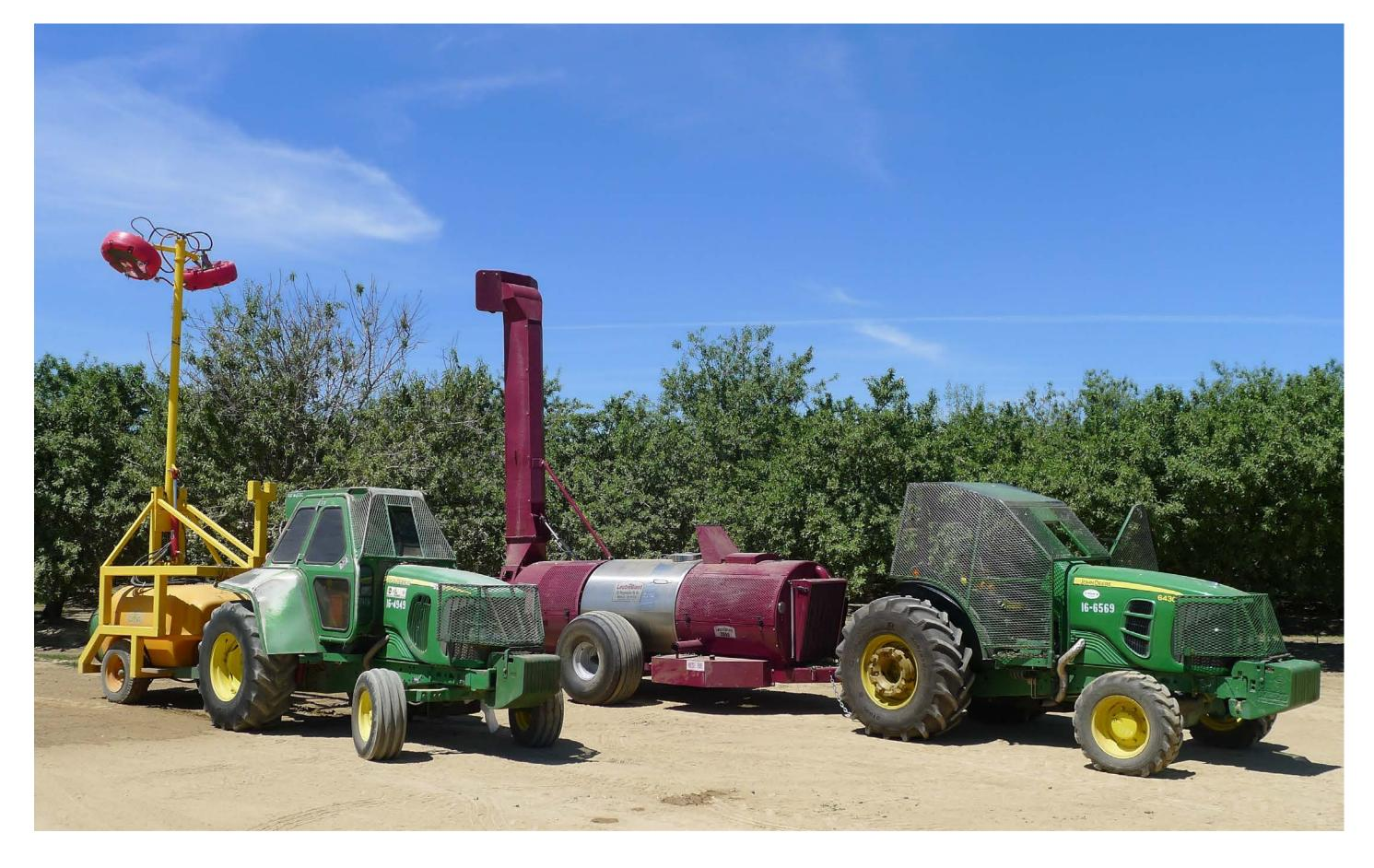
The modified test sprayer (left), along with a tower sprayer, positioned in the commercial orchard for hull-split spray testing. Split (two dates) applications were made. Mechanical durability and compatibility with commercial demands was proven. Pest control efficacy data are pending analysis.
