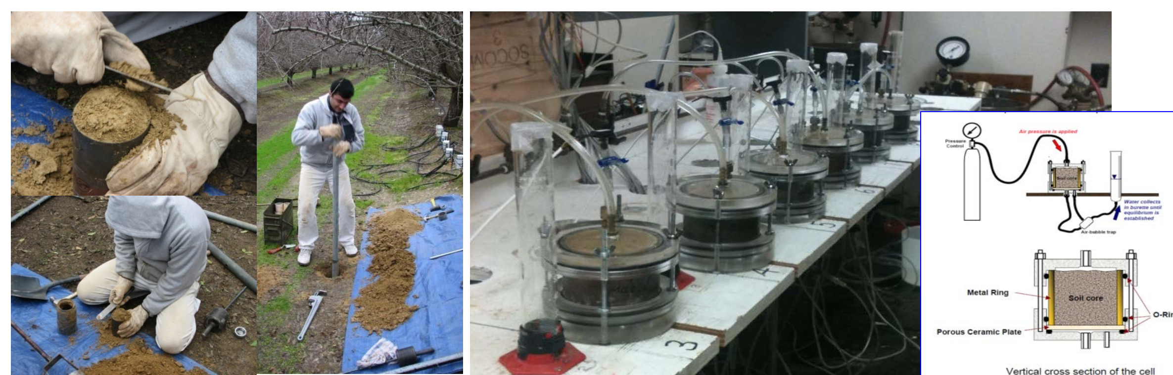
Fig. 6. Collecting undisturbed soil sample in the field and measurement of soil hydraulic properties of undisturbed soil core in the laboratory (outflow method - Tempe cell)
