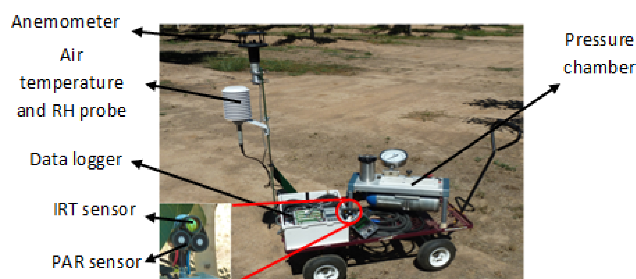
Fig. 1. Mobile sensor suite and pressure chamber used during data collection in an almond orchard.
