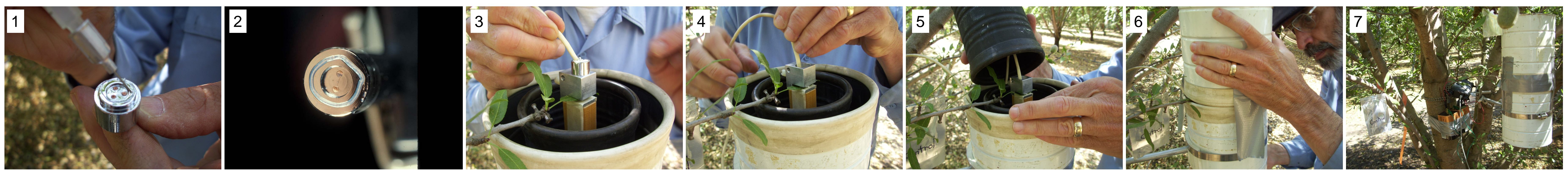
Figure 2. Steps in the process of sealing an in-situ psychrometer to an almond leaf. The chrome face of the psychrometer must be lined with a thin strip of non-toxic silicone grease (1 and 2), then placed in an aluminum block, which fixes the psychrometer against the leaf (3 and 4). The leaf surface in the area covered by the psychrometer must be gently abraded in order to have good vapor exchange between the leaf and the psychrometer (not shown). The psychrometer and attached leaf are enclosed in metal cans which dampen thermal fluctuations (5 and 6), which are relatively bulky and must be supported by clamping to a nearby scaffold (7). During the insulation assembly, it is critical that the leaf is not disturbed with sufficient force to disturb the psychrometer/leaf seal or damage the leaf or leaf/stem connection.
