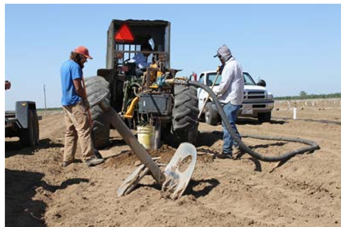
Figure 1. Redesigned steam-injection auger for treating almond tree planting sites. A 24-inch diameter auger (in use) and a 36 inch auger (foreground) were tested in trials throughout the San Joaquin Valley, CA.
