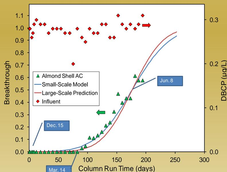
Figure 3. Column studies demonstrated that 100% of the DBCP could be removed for at least 14,000 bed volumes (90 days of operation), and that a mathematical model allowed predictability of large-scale systems.
