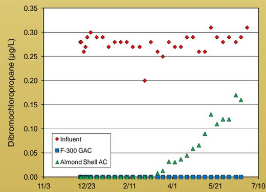
Figure 2. DBCP concentrations of Well # 184 influent, and effluents from experimental columns.
