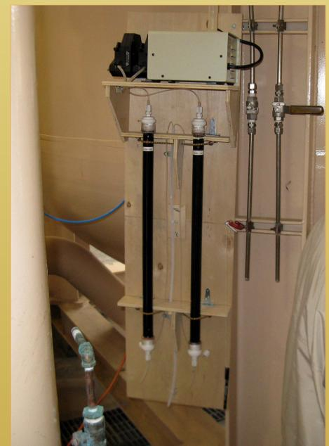
Almond shell GAC and F-300 experimental columns mounted on the sampling ports of a Model 12 vessel.
