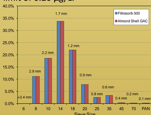
Figure 1. Particle size distribution of commercial activated carbon (F-300) and the GAC made from almond shells.
