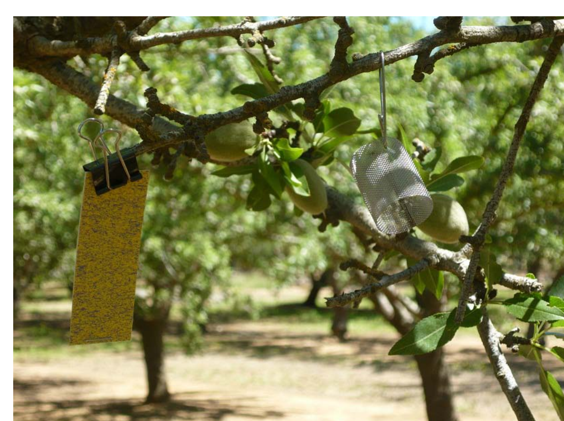
Figure 5. Deposition on water sensitive paper within the low canopy after hull-split treatment (note adjacent mesh cylinder).
