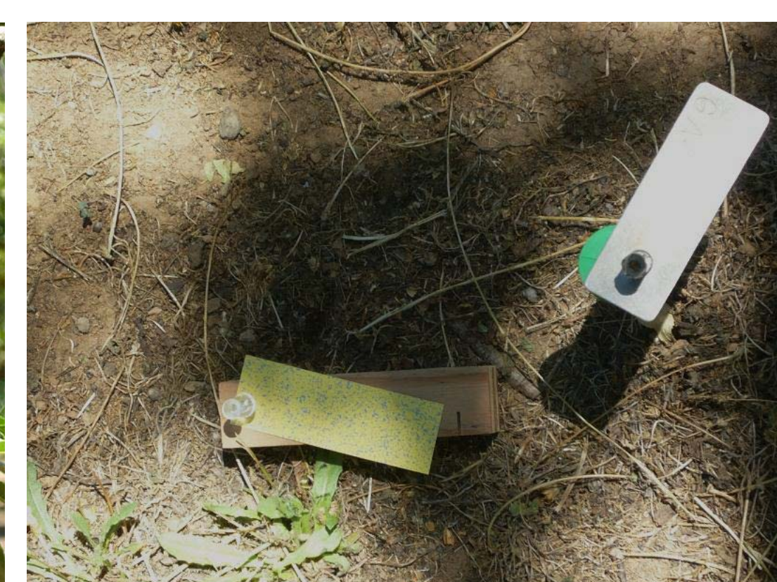
Figure 6. Ground deposition on water sensitive paper along the tree line (note adjacent steel plate media).
