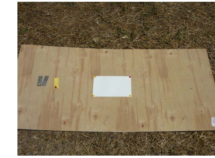
Figure 8. Drift sedimentation platform with alpha-cellulose sheets (9 in. x 6 in.), water sensitive paper (1 in. x 3 in.) and steel plates (1 in. x 3 in.).
