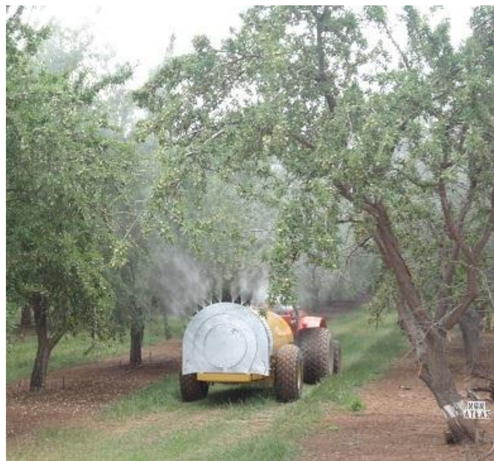
Experiment 2: Spraying tall almonds late spring, 2011. Air-O-Fan GB36 PTO sprayer; 110 gpa; 150 psi; 2 mph; micronutrients in sprayer as tracer. Question: Will using many, small droplets (2x nozzles) deposit more spray material in the tree tops? Answer: NO.
