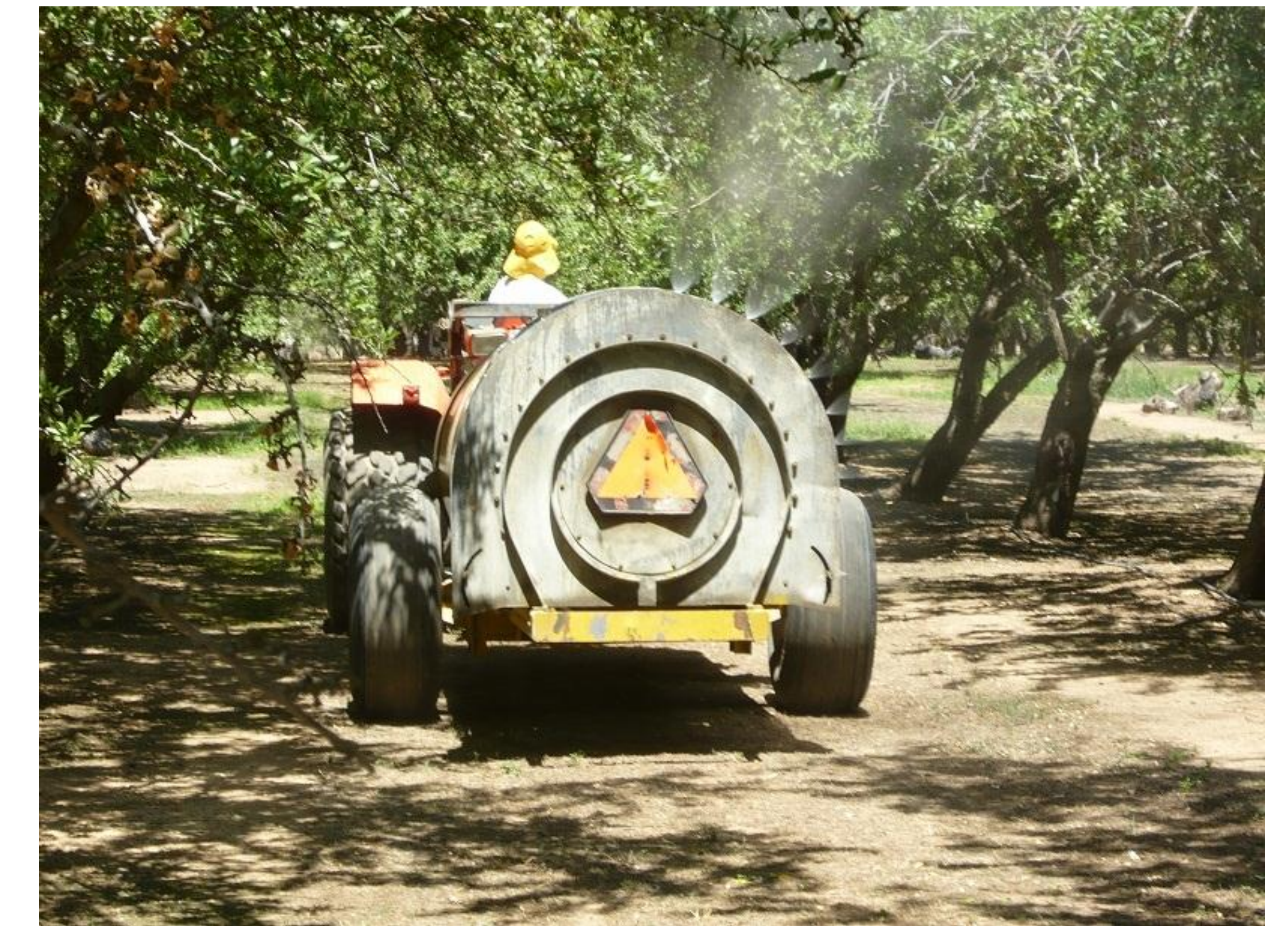
Experiment 3: Spraying almonds during hull split 2011 Air-O-Fan GB36 PTO sprayer; 100 gpa; 150 psi; Altacor (4 oz/acre), micronutrients in sprayer as tracer. Question: Will directing more pesticide towards the tree tops and driving faster (2.5 mph) give the same NOW control as the usual nozzle set up (2/3 of pesticide through top half of nozzles) and slower tractor speed (1.8 mph)? Answer: NO.
