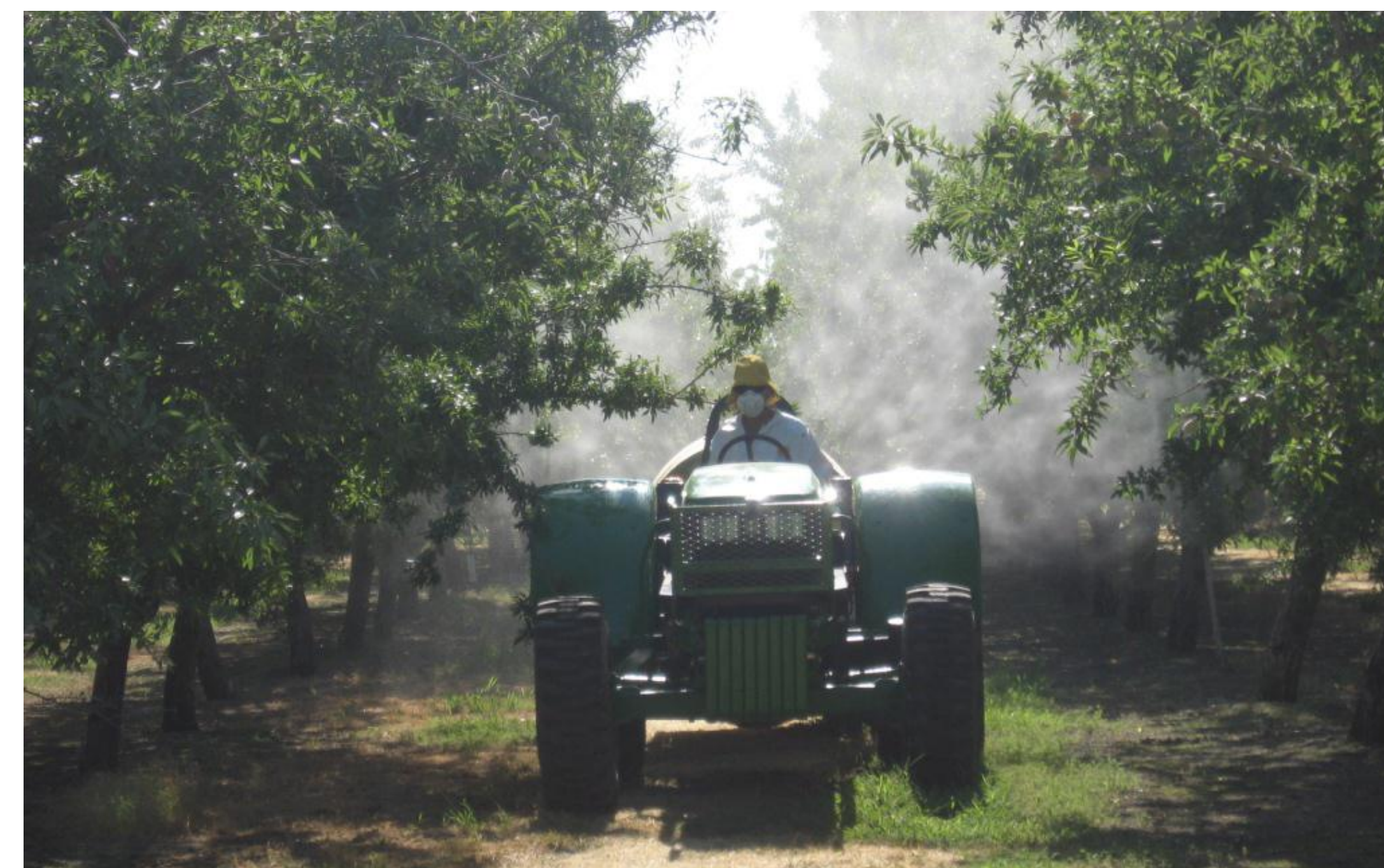
Experiment 1: Hull split spray, 2010. TurboMist S30 PTO sprayer; 150 psi; 2 mph; Brigade WSB @ 1.5#/acre. Question: Will spray volume differences (50 gpa vs 100 gpa) effect NOW control? Answer: NO.
