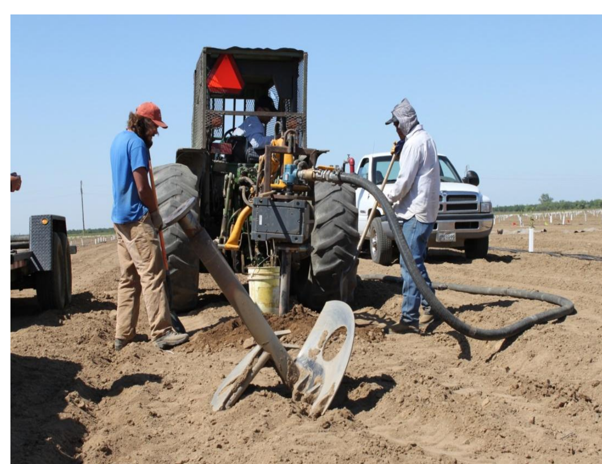
Figure 3: Redesigned steam-injection auger for treating almond tree planting sites. A 24-inch diameter auger (in use) and a 36 inch auger (foreground) were tested in trials near Delhi and Wasco, CA.
