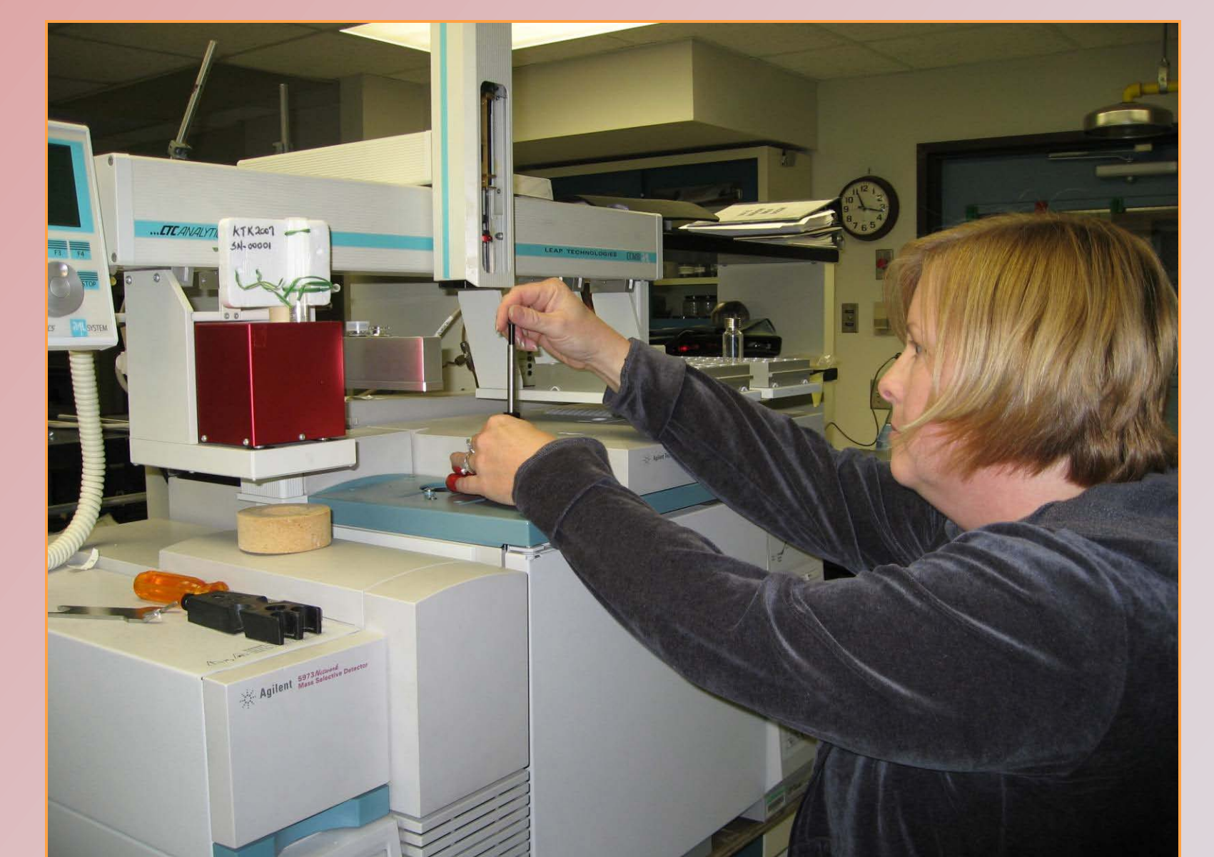
A gas chromatograph equipped with electron capture detection is used to analyze halogenated compounds, such as DBCP in water.
