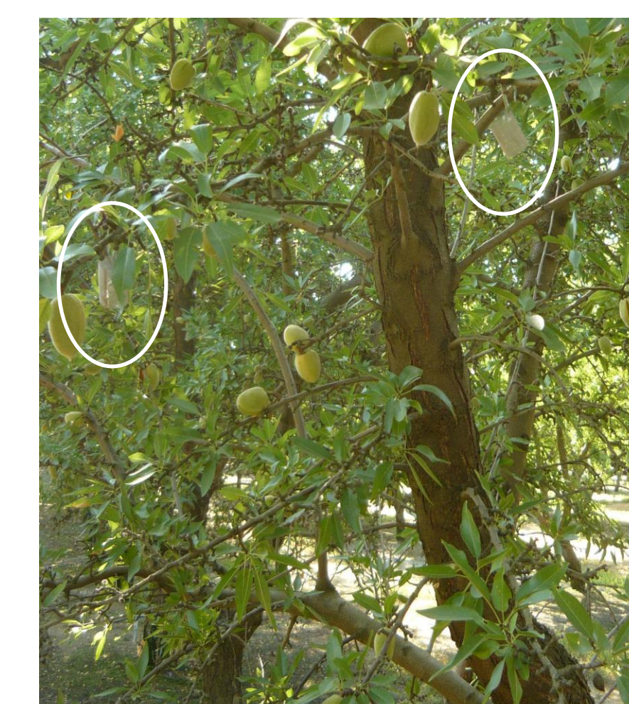
Figure 8. Spray deposition media in tree: stainless steel mesh cylinders (1 in dia., 3 in long).
