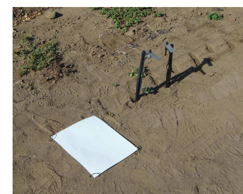
Figure 5. Drift deposition media: Mylar sheets (8 x 12 in) and stainless steel plates (1 x 3 in).
