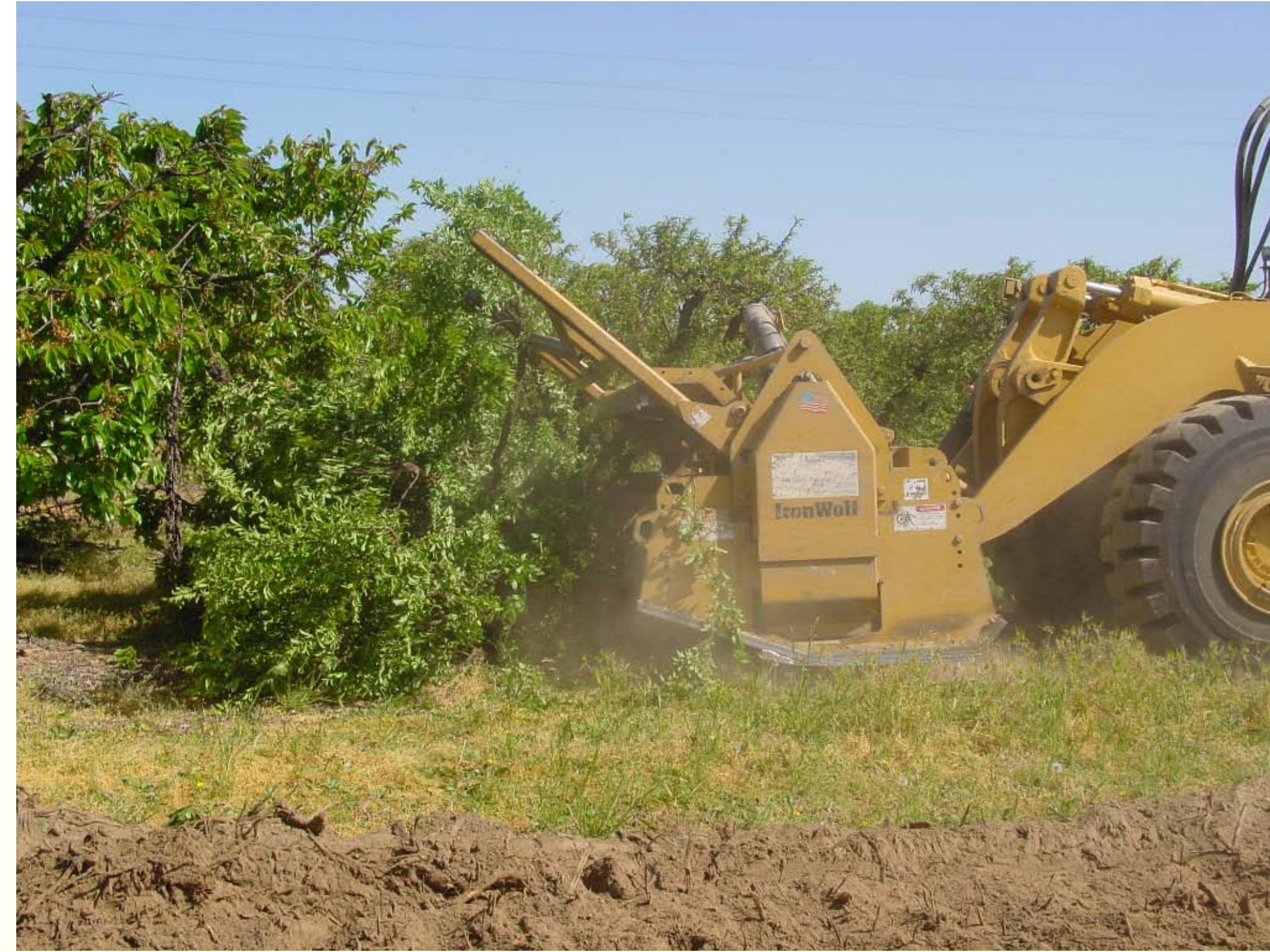
Tree being pushed over and ground in place by the 'Iron Wolf'
