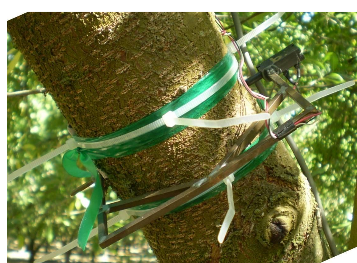
Figure 7. (Micro) dendrometer attached to a primary scaffold.
