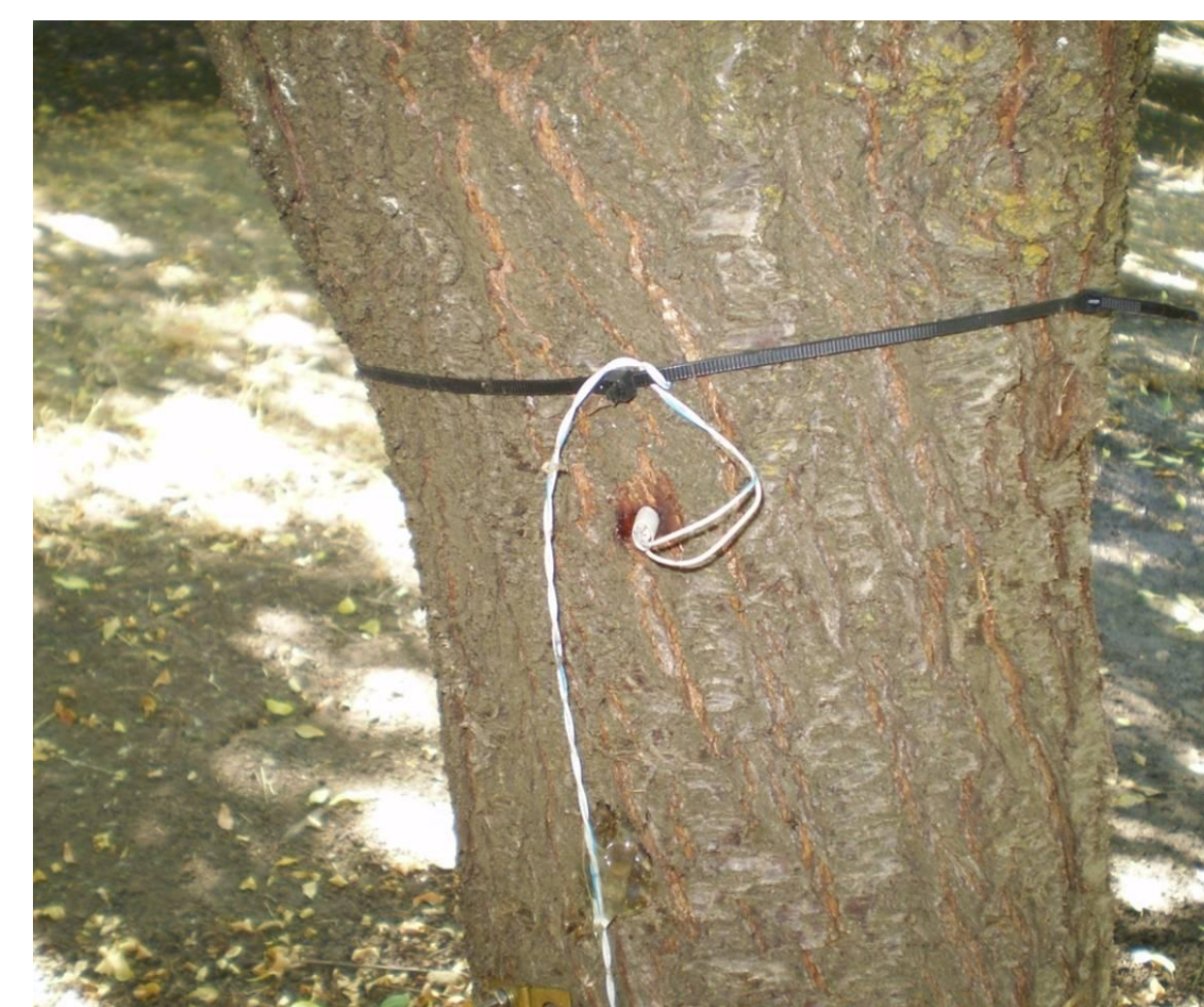
Figure 1. Phytogram sensor for automated and continuous measurement of sapwood water content, installed in the tree trunk.
