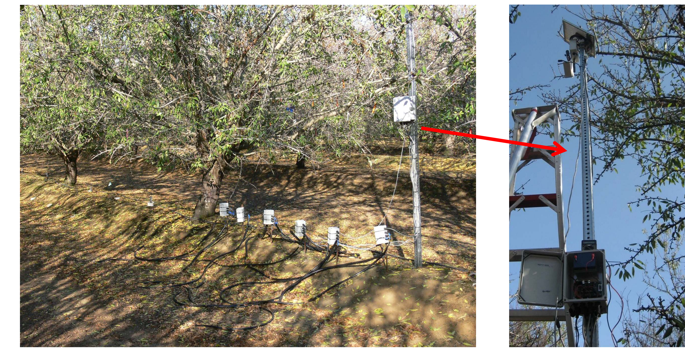
Fig. 6. A schematic of the tensiometer installation at different layer in the soil profile.
