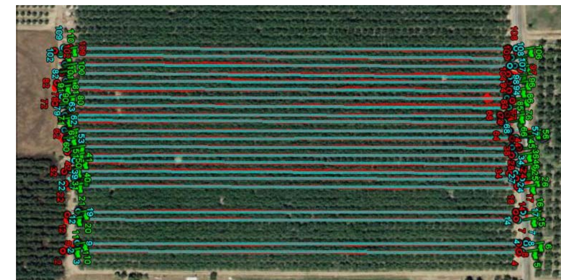
Fig. 2. Aerial image of SCRI Arbuckle almond trial mapped with the mobile lightbar. Numbers on image represent points at which full sun and GPS readings were taken. Blue lines are connecting two full sun readings done outside of orchard for each row and red line is actual GPS trace through orchard.
