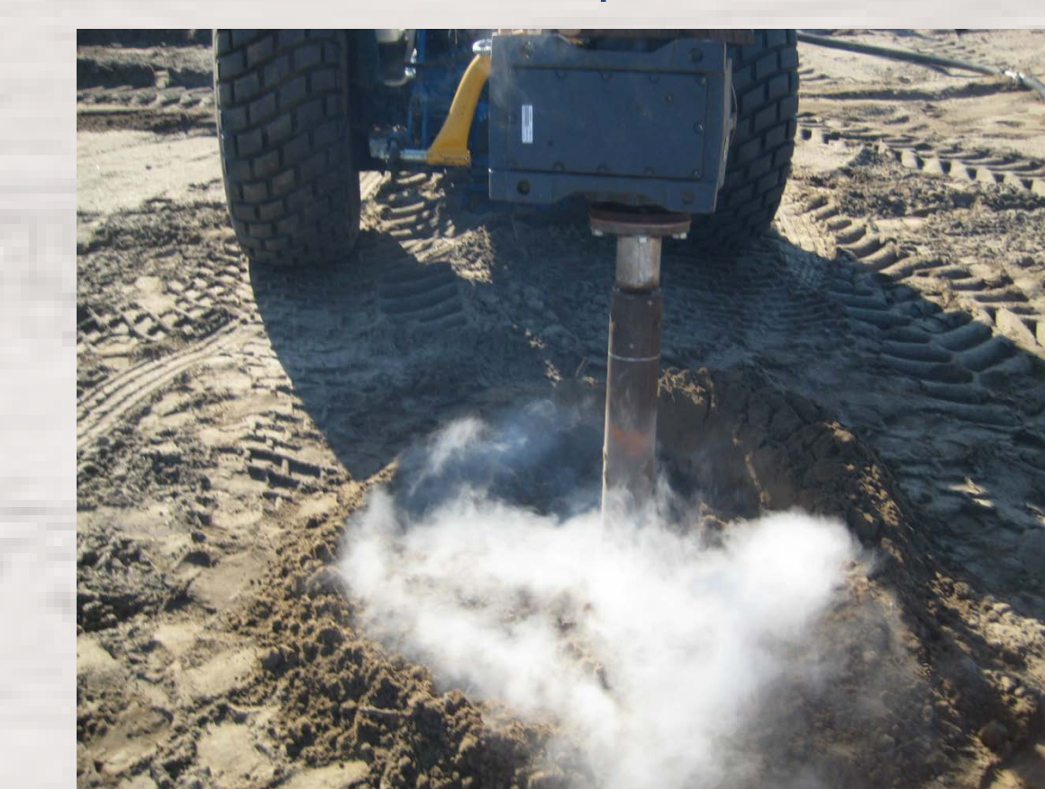
Figure 5: A modification to the steam-injection auger may be needed to minimize untreated soil being returned to the tree site after steam injection.
