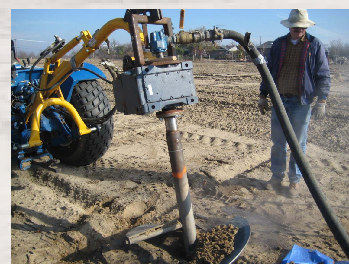
Figure 3: Testing of the redesigned steam injection auger in an almond replant trial in near Delhi, CA in December 2010. Steam was injected for 6 minutes in 36 inch diameter tree sites and for 2.5 minutes in 24-inch treated sites.
