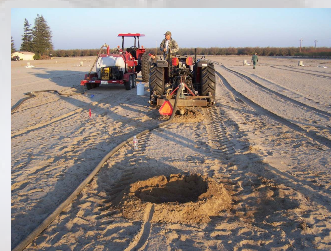
Figure 2: Testing of the prototype steam injection auger in an almond replant trial in near Livingston, CA in December 2009. Steam was generated using a diesel-powered boiler and steam was injected for four minutes in each hole as the soil was agitated.
