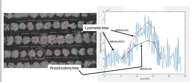
**Figure 3.** (Left) Lidar scan of the lysimeter tree (labeled '9') and nearby Nonpareil and pollinizer trees. (Right) measured and modeled ET for the lysimeter tree and for a nearby Wood Colony tree (labeled '15') for the weather conditions on the day of the Lidar scan (October 11, 2017). The modeled values are for intervals of 2h, whereas the measured lysimeter values are for 10 minute intervals, and hence exhibit much more random variation.
