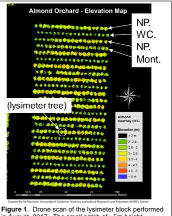
**Figure 1**. Drone scan of the lysimeter block performed in August, 2017. The small patch of >5m height reading accurately corresponds to an ET tower in the canopy of the tree that is adjacent to (east of) the lysimeter tree.
