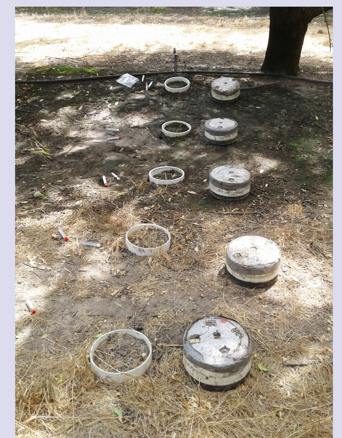
Figure 1: General setup of static gas chamber collars in orchard rows.
