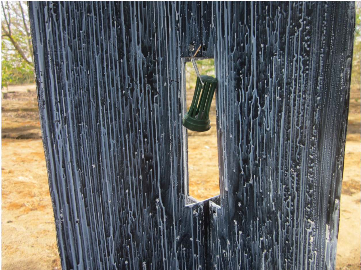
Figure 8. Close-up of a crossvane panel trap coated with fluon. The hanging basket in the center of the trap contains the pheromone lure
