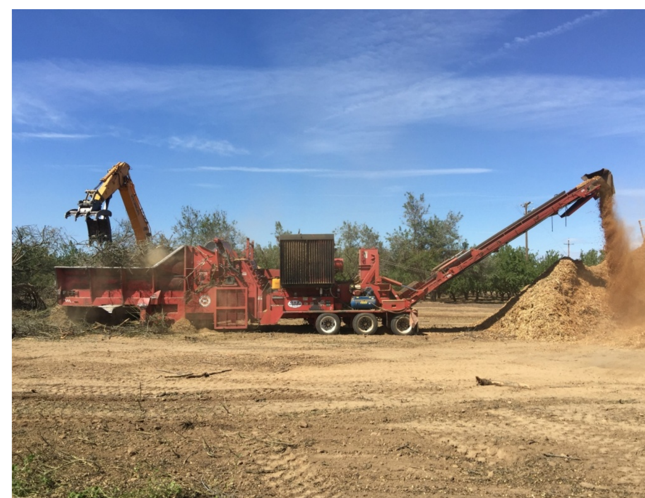
Figure 3. The Morbark horizontal chipper was used to chip up almond trees at Agriland for comparison with the Iron Wolf.
