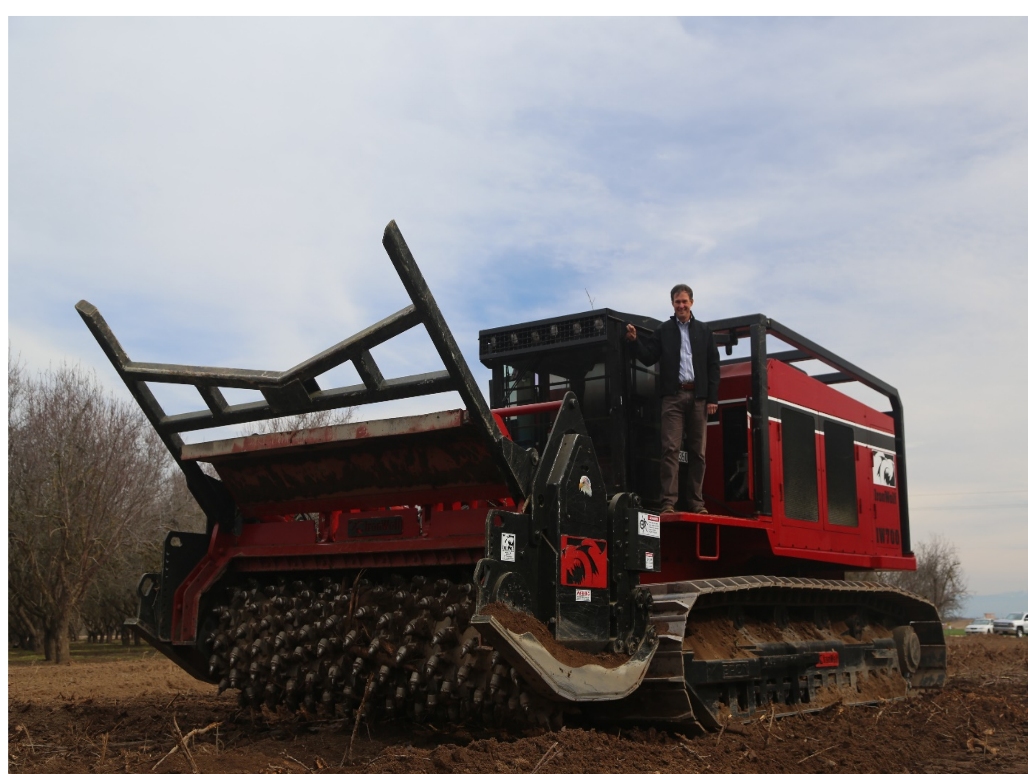
Fig. 2. The 'Iron Wolf' 700 B, a 50-ton rock crusher, pushes trees over going forward while grinding branches and trunks. Then going in reverse the Iron Wolf can incorporate the wood, at a rate of 2 acres per day and at a cost of approximately $1,500/acre.
