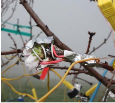
Figure 6. Bud heating devices allowing to break dormancy in buds. 29 January 2016
