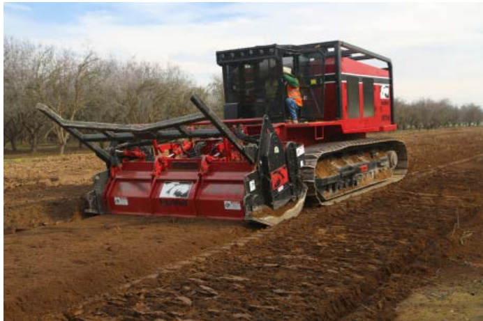
Figure 2. The 'Iron Wolf' 700 B, a 50-ton rototiller, built to remove forests and crush rock, was used to grind up almond trees at Agriland Farming in Chowchilla. In the photo the Iron Wolf is going in reverse and incorporating the ground up trees.
