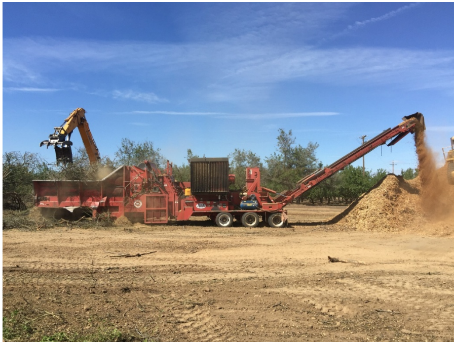
Figure 3. The Morbark horizontal chipper was used to chip up almond trees at Agriland for comparison with the Iron Wolf. These chips were spread out on the soil surface in the whole orchard recycling with wood chips treatment (WOR-C), then cultivated back into the soil with a stubble disk.
