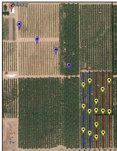
Figure 1. Wireless mesh network located at Nickels Soil Lab., where the red mark corresponds to the gateway, blue marks correspond to the repeaters and yellow marks correspond to ekonodes to which leaf monitors and latching solenoid valves are connected.
