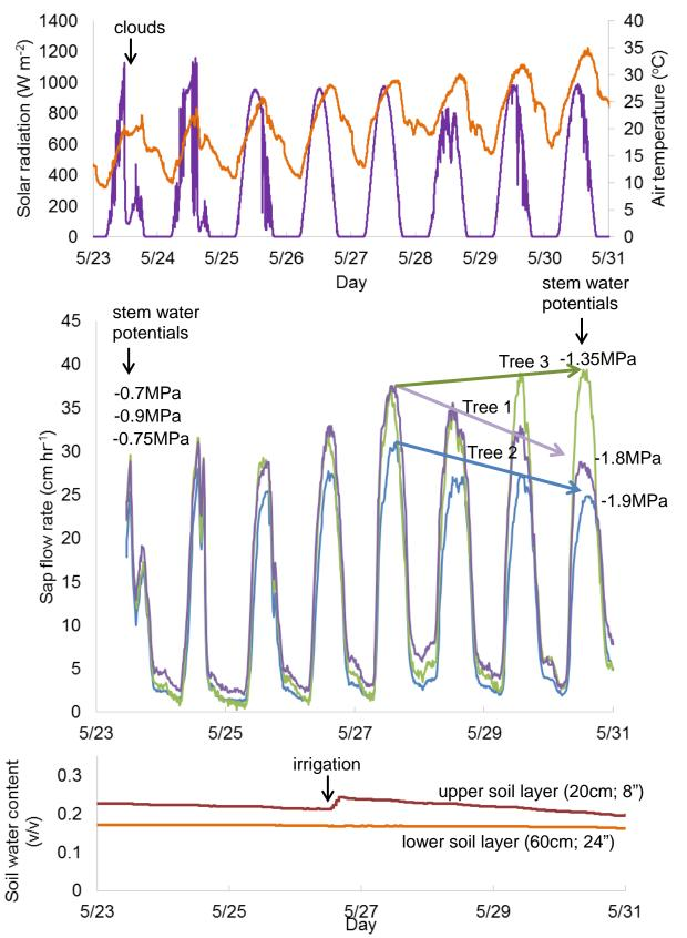
Figure 8. Illustrative sap flows during a hot period with one irrigation event. Volumetric soil water contents were average values for two depths across the orchard.
