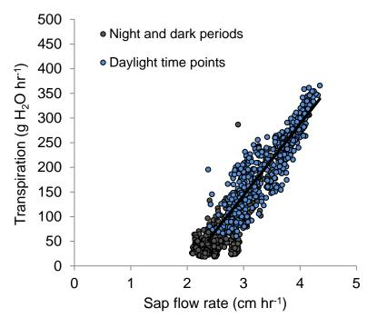
**Figure 5.** Correspondence of weighing lysimeter measurement of transpiration, and sap flow measurement. These data represent a two-week period during which measurements were made every 15 minutes. A zero flow correction was not performed for this tree, meaning that non-parallel temperature sensors resulted in the prediction of 2 cm hr<sup>-1</sup> flow rate at a measured transpiration of zero.
