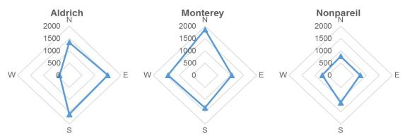
**Figure 3.** Illustrative cumulative daily flow rates (cm hr<sup>-1</sup>) for three trees of three varieties showing different sap flows with direction in tree. The variation partially reflects the variation in water conductive sap wood thickness around the tree. These data represent one tree per almond variety, and thus are not representative of that variety.
