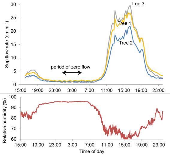
**Figure 7.** Illustrative sap flows measured during period of zero flow – a rainy night. The sap flow rates shown above are for the Combined method where the sensor spacing was calibrated for zero flow.
