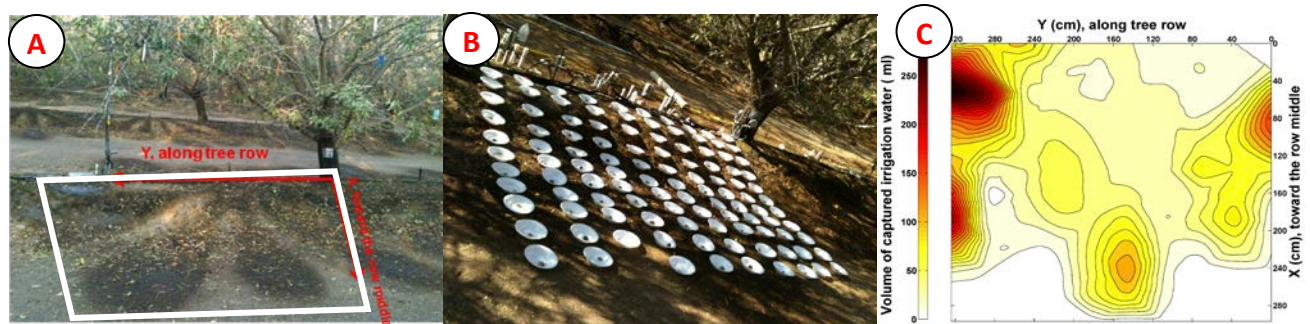
Figure 5. Measurement (a and b) of water application uniformity and uniformity pattern (c) for the fanjet (1 hour volume measurements).
