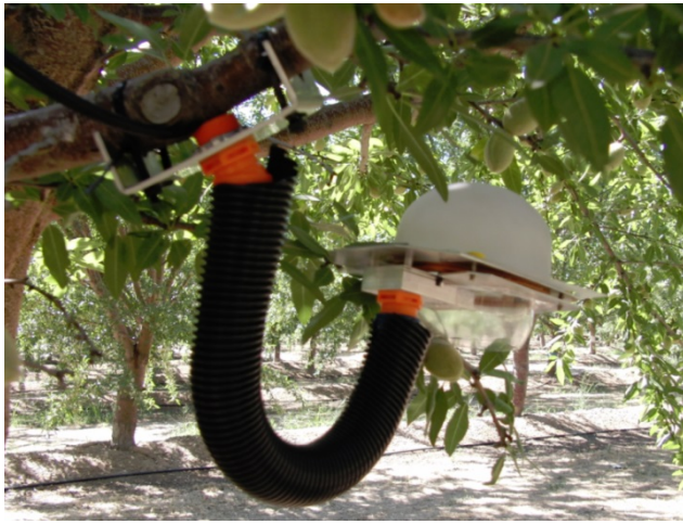
Figure 7(a): Leaf monitor installed in almond.
