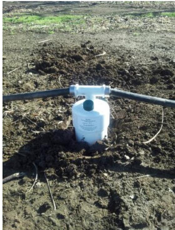
**Figure 5.** Microfertilization dosetrons used in the HFLC subplots.
