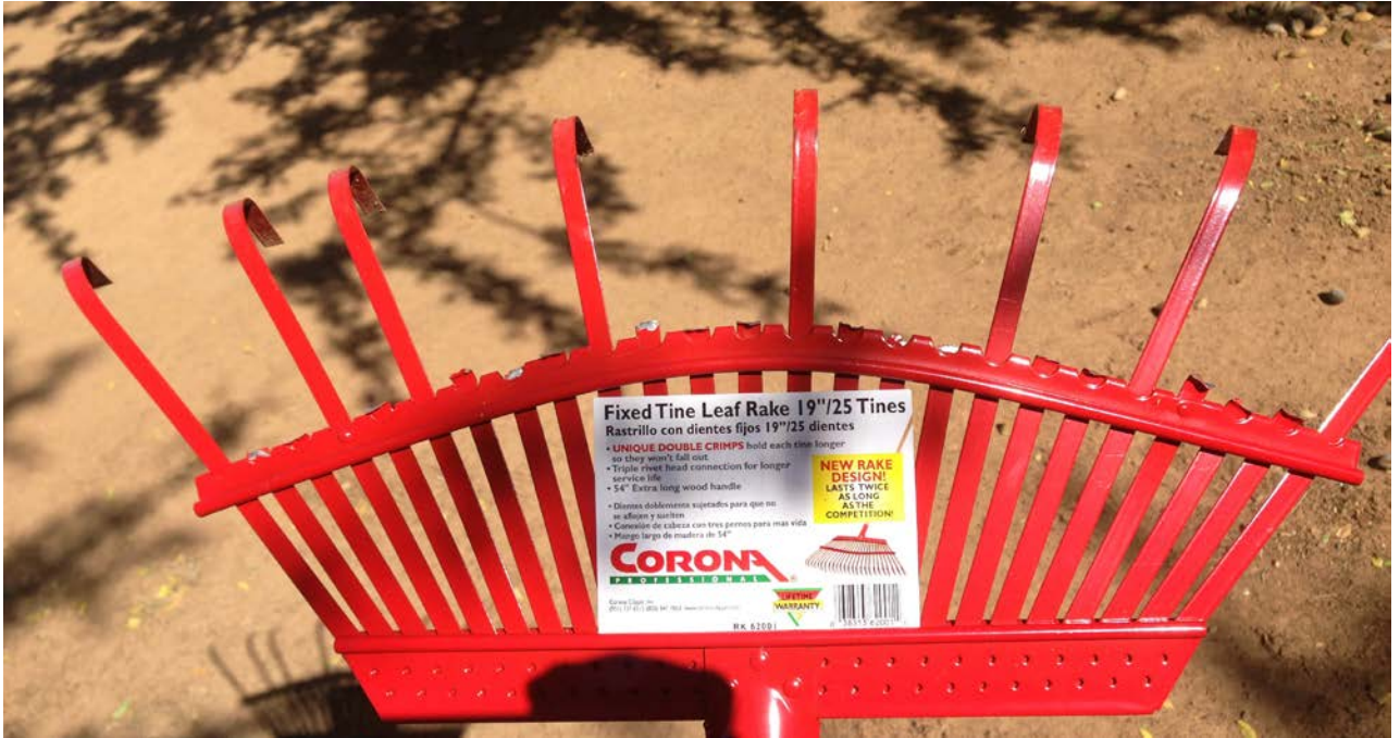
Figure 2. Modified rake to roll wet nuts. October 1, 2013.
