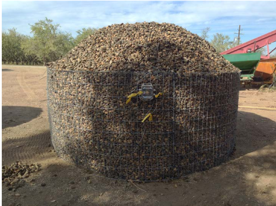
Figure 4. Completed experimental stockpile with datalogger for storing temperature data in upper center of the photo. November 1, 2013.
