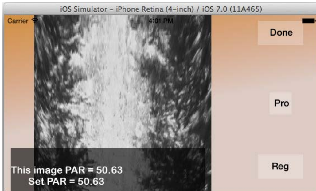
Figure 10. Image showing the image corrected for perspective with the estimated midday canopy light interception shown.
