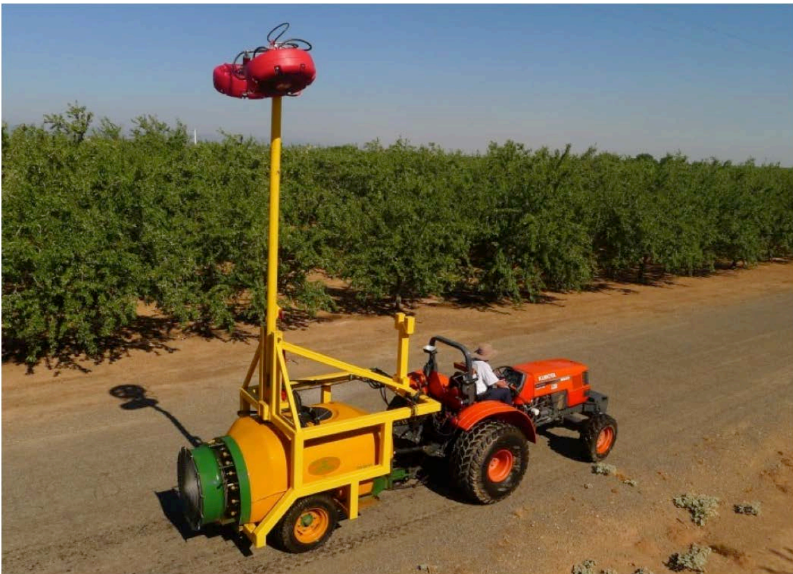
Figure 3. Completed retrofit sprayer design as deployed for field testing.
