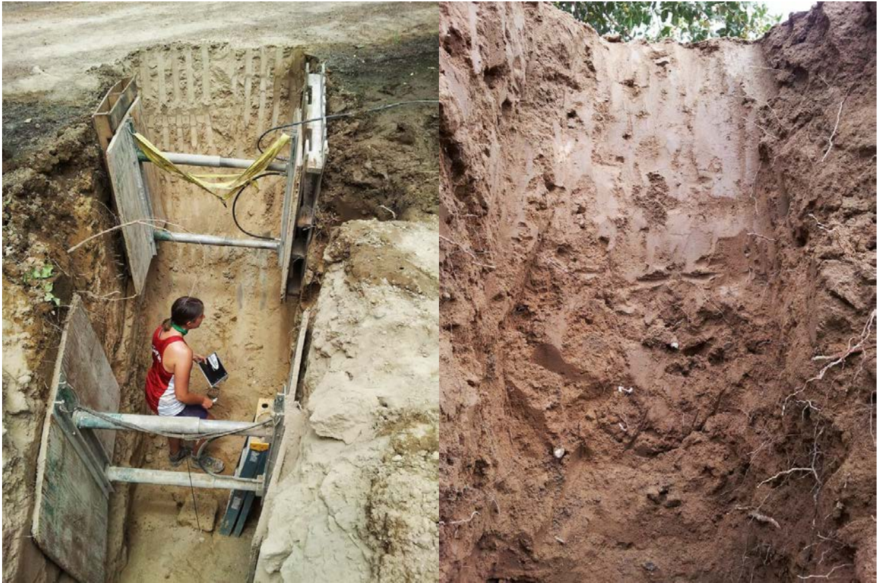
Figure 3: Shown in the left panel is Ms. Nicole Niehues, MSc. student in the UC Davis Soils Biogeochemistry Graduate Group who is collecting horizon specific soil bulk density samples. In the right panel is an example of the lack of horization in a sandy loam soil in a pistachio orchard and roots on the wall profile that allow us to designate an appropriate root zone for future instrumentation of the site for intensive monitoring of water and NO 3 - solution movement through the vadose zone.
