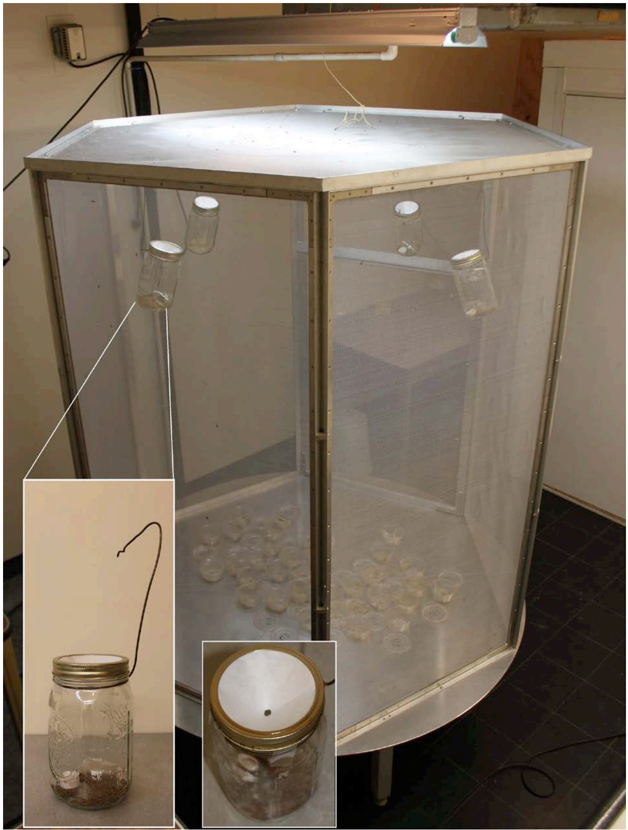
Figure 1. Bioassay cage with insets pictures of the capture jars. The cage is 1.5 m high and 1.5 m across. Virtually no males are captured in any treatment that we have tested to date and empty jars (negative controls) captured ca. 1% of the released moths (0-2 moths per replicate).
