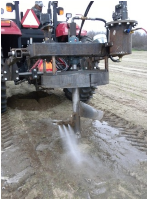
Figure 1: The liquid injection auger that has been used within the trials to inject and mix the product within the root zone.
