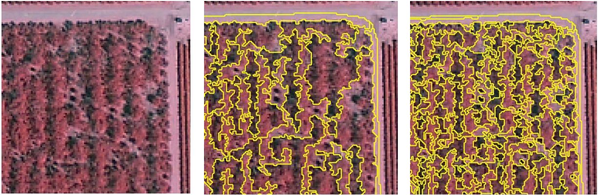
Figure 2. NAIP imagery pixels (left); low homogeneity (higher variance) objects (center); high homogeneity (lower variance) objects (right)
