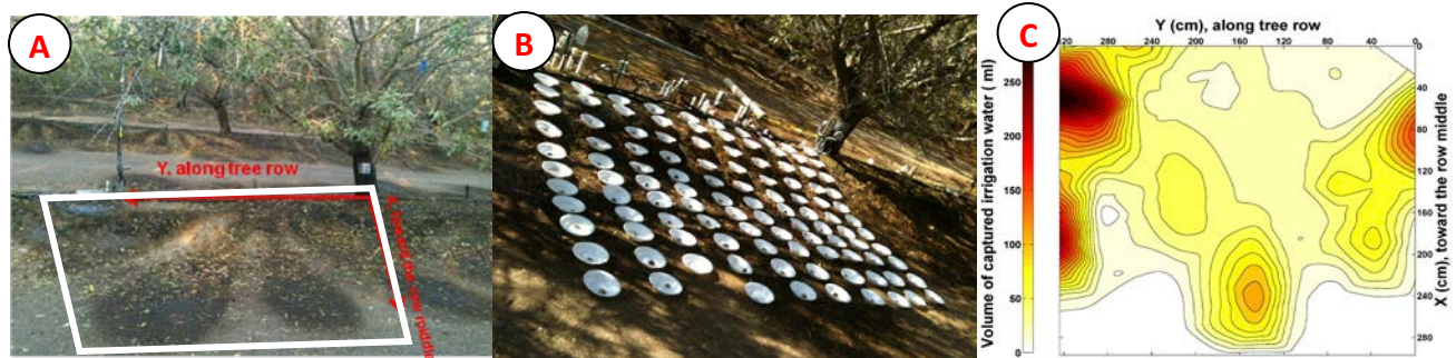
Figure 4. Measurement (a and b) of water application uniformity and uniformity pattern (c) for the fan jet (1 hour volume measurements).
