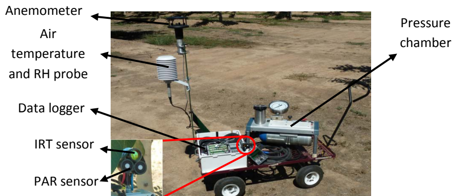
Figure 2. Mobile sensor suite and pressure chamber during data collection in an almond orchard.
