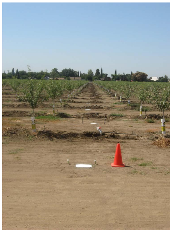
Figure 3. Drift sedimentation transect south of the test orchard (perpendicular to the primary spray direction).
