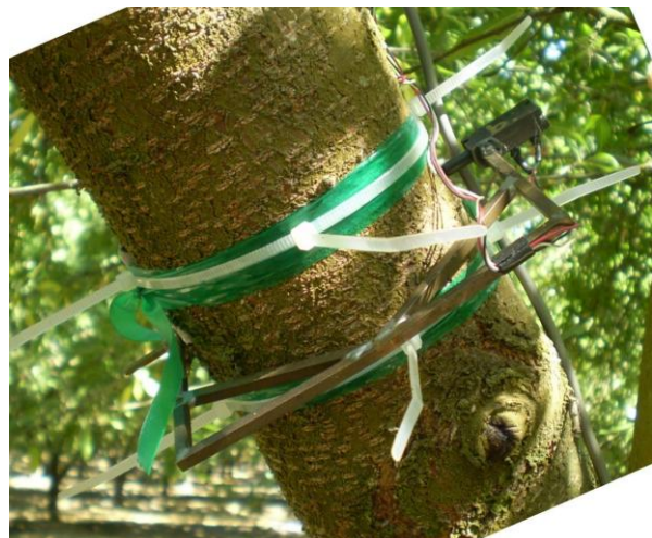
Figure 2. (Micro) dendrometer attached to a primary scaffold.
