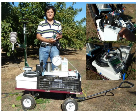
Figure 2. Sensor suite used to determine plant water status.
