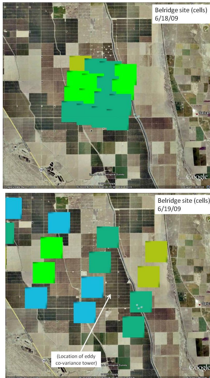
Figure 10. Aerial view of the experimental site on two consecutive dates, showing the high degree of variability that occurs in the location of data points (cells) used by the RSET program.
