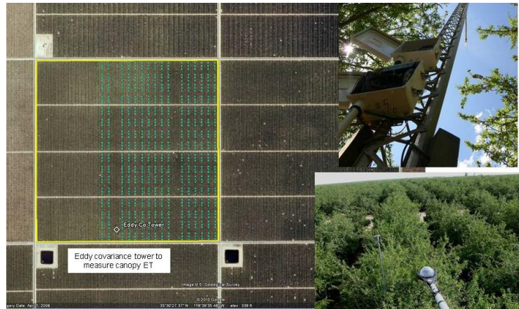
Figure 1. Experimental site at Belridge and the instrumentation used to measure orchard ET.
