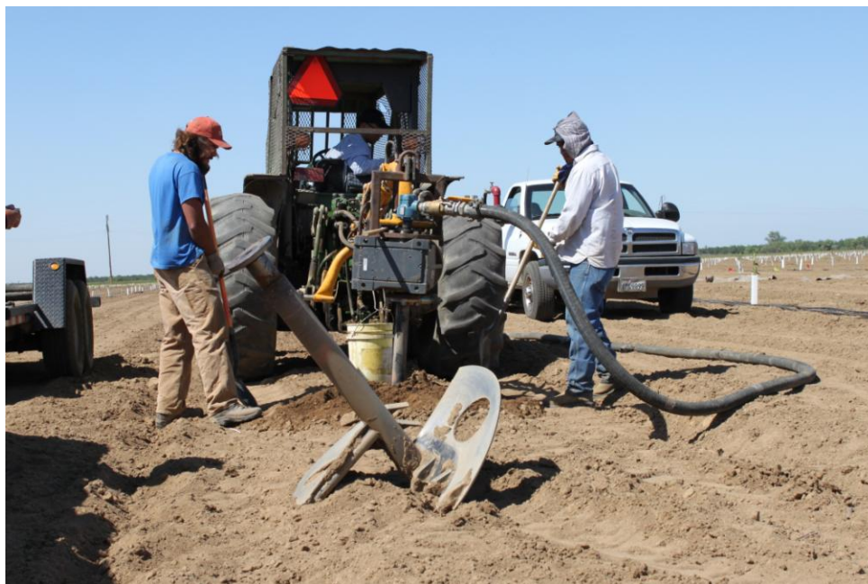
Figure 1. Redesigned steam-injection auger for treating almond tree planting sites. A 24-inch diameter auger (in use) and a 36 inch auger (foreground) were tested in trials near Delhi and Wasco, CA.
