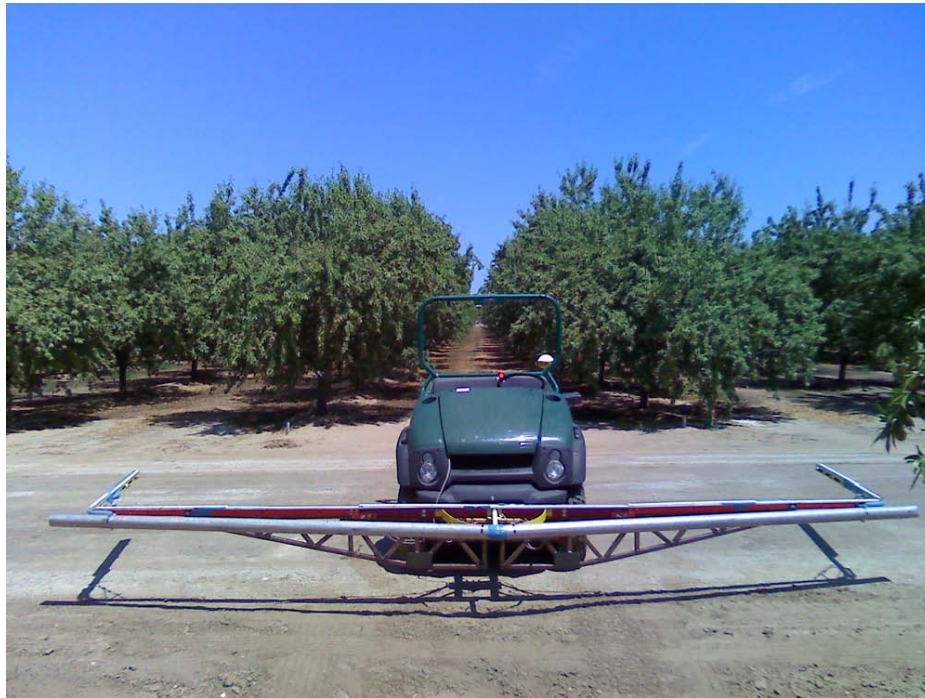
Figure 1. Current design of Kawasaki Mule mounted lightbar after summer 2009 modifications showing adjustable end section and branch bumper on front designed to aid in pushing through orchards with many low overhanging branches.
