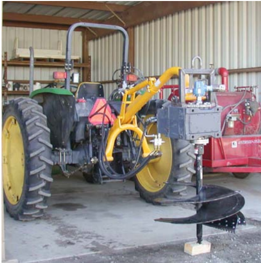
Figure 1. . Finished auger fabrication on Nov. 7, 2009. Shown are the auger, gear box, 3-pt. connection and hydraulic drive.
