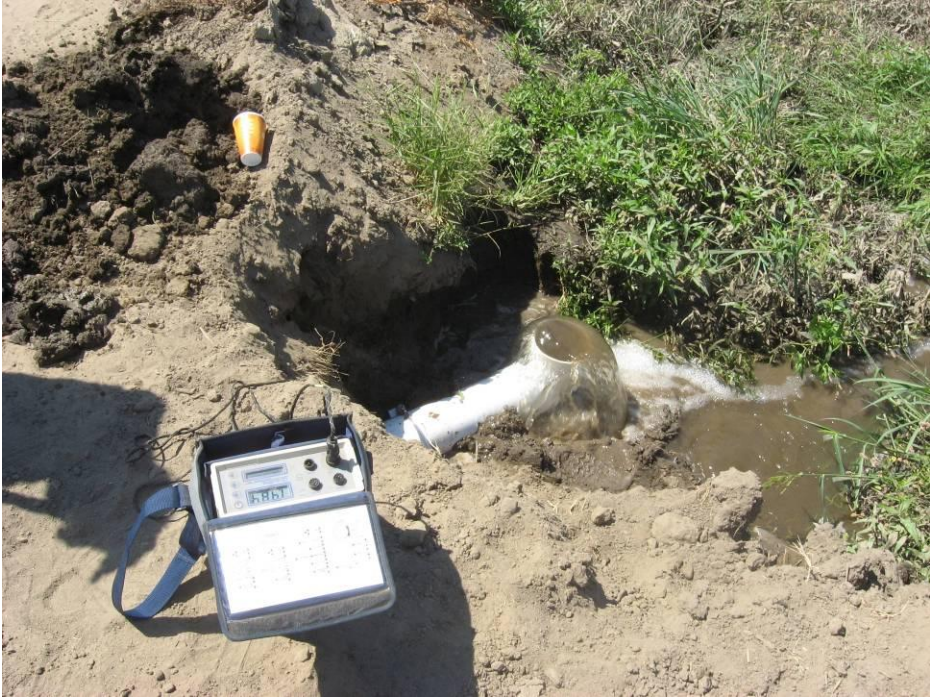
Figure 8. Doppler Flow Meter at Entrance to Sediment Basin
