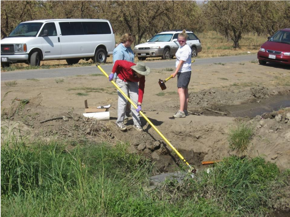
Figure 9. Sampling Residues with Swing Sampler at Entrance to Sediment Basin
