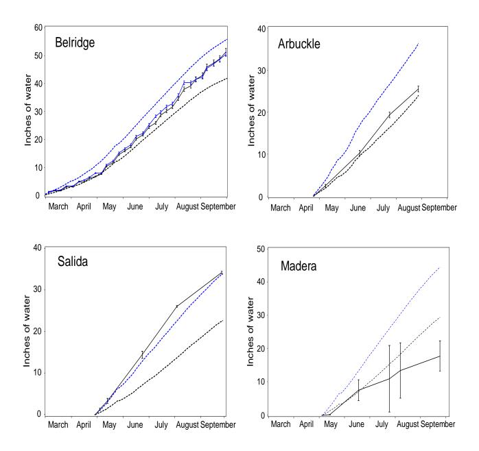
**Figure 1.** Cumulative inches of water applied during the observation period (starting with water meter installation, solid lines), and upper (full cover) and lower (clean tilled) CIMIS estimates of irrigation requirement (Etc-rain, dashed lines). Error bars are ±2 SE and indicate variation in the water applied through two independent lateral lines.
